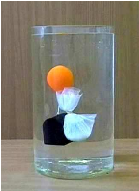
Fig. 2: The rubber balloon with attached ballast weight and salt bag
